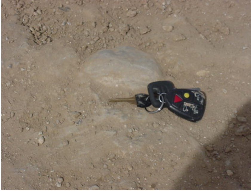
Figure 1: (a) Example of unacceptable clod sizes and protruding elements and (b) example of unacceptable protrusion size
