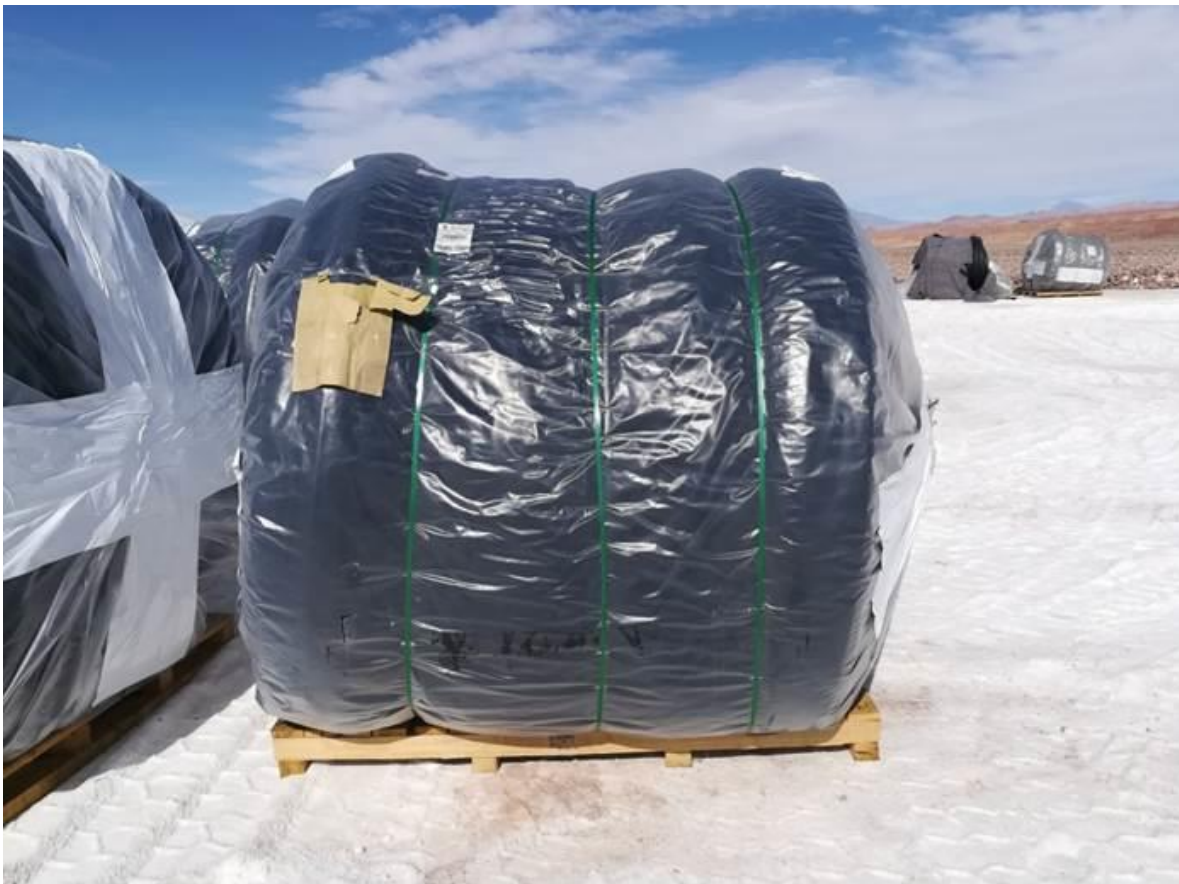
Figure 2. Uneven rolled panel prior to deployment.
