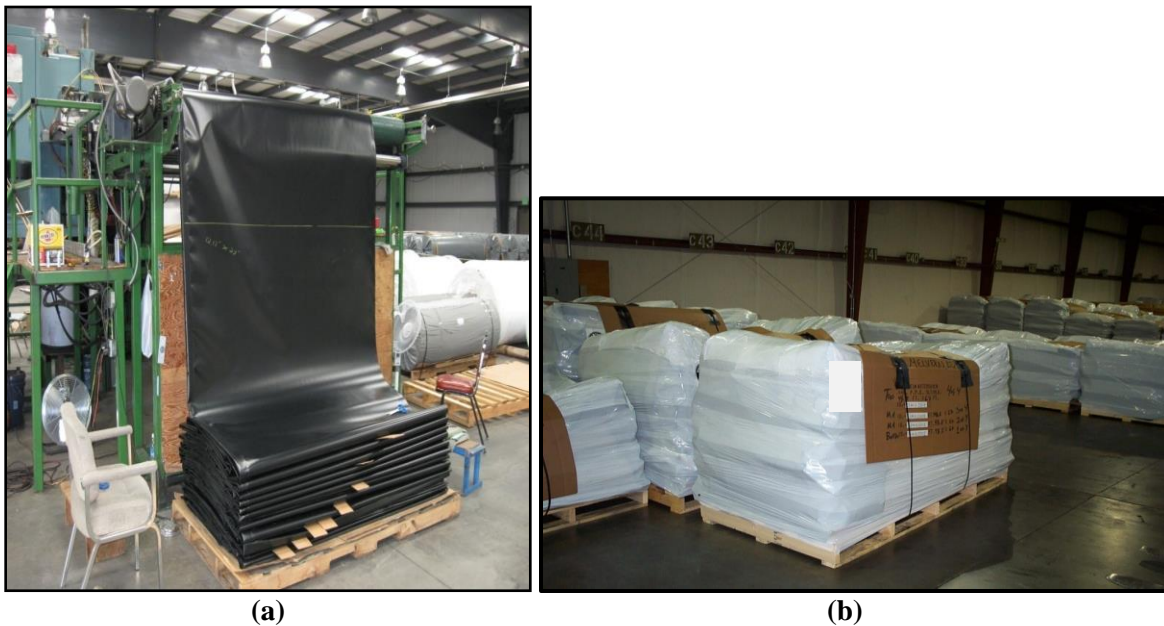
Figure 3. Photographs of: (a) factory fabricated geomembrane panel being accordion-folded onto a wood pallet for shipping and (b) accordion-folded panels wrapped for shipping.
